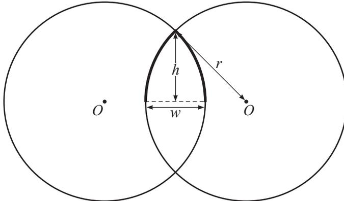
The equal arcs are parts of the circumferences of two identical circles both of radius  $r$  metres. The base of the arch is on the line joining the centres of the two circles. The height is on the line of symmetry of the arch.
