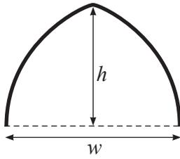
This arch is made using two equal arcs.
